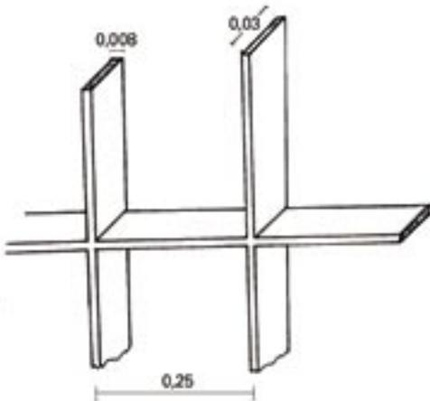
*Details of bar spacing.**Figure 8. Security fence construction.***4.3.4 Water barriers**
