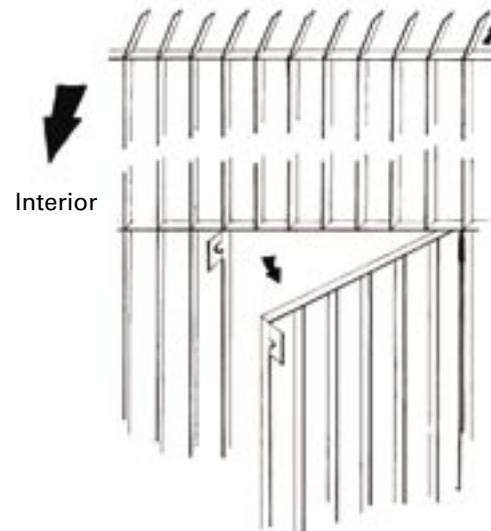
*Detail: orientation of the door and the ends of the bars.*
